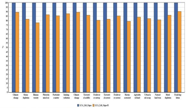
Method: ReCiPe Endpoint (H) V1.12 / Europe ReCiPe H/A / Characterization / Excluding infrastructure processes / Excluding long-term emissions Comparing 1 p 'LCA\_Lift\_Gigas' with 1 p 'LCA\_Lift\_Gigas-R';
